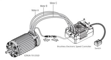
M4 mounting screws are needed there, and the mounting holes are 7mm in depth, before installing the motor on the vehicle, please carefully confirm whether the specification of the screws is appropriate according to the thickness of the motor mounting plate to avoid damage to the motor due to too long screws.
